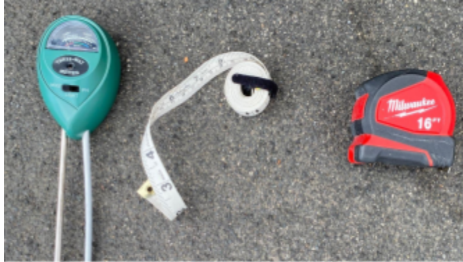
Figure 9. Tools used for data collection. (From left to right) 3-way soil meter, sewing tape, tape measure.
